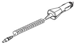
The input voltage range is from 11 to 32V DC, negative grounding. Avoid prolonged charging with the Rapid Cigarette Lighter Charger (LCH-9) when the car engine is not running; this could cause your car battery to drain. Note also, that in some cars, the cigarette lighter plug is not provided with electricity if the ignition is not switched on.
